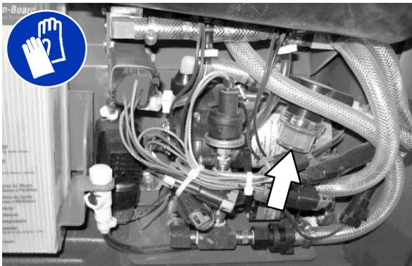
**SUBSTITUIR OS FILTROS DO SISTEMA FaST**
